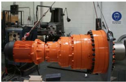
Above: A Brevini gearbox and motor awaiting installation on a HotRot 1811
