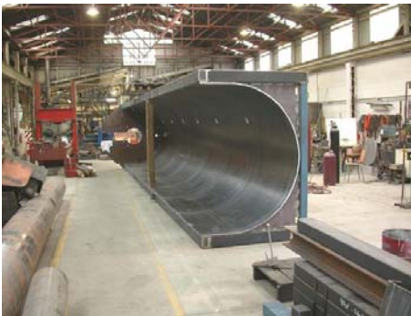
Above: A HotRot 1811 hull under construction in the Mace Engineering workshops
